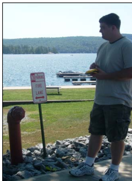
Marty uses the Trimble GPS unit to locate a dry hydrant. The data will be used to create a map database.
