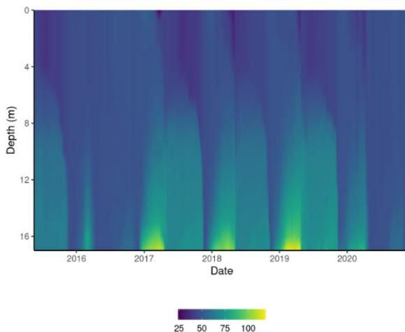
Figure 3. Chloride (mg/L) from vertical profiles collected at 1-m intervals at the deepest part of the lake from 5/18/2015 to 12/31/2020. Lighter color denotes higher concentrations of chloride.
