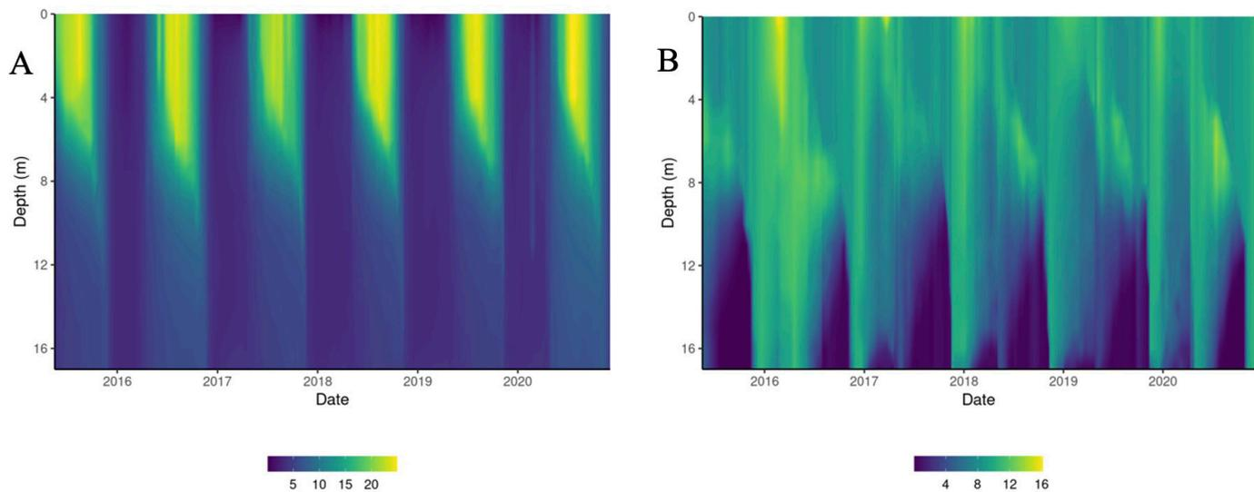
Figure 2. Temperature (°C) (A) and dissolved oxygen (mg/L) (B) from vertical profiles collected at 1m intervals at the deepest part of the lake from 5/18/2015 – 12/31/2020. Lighter color denotes higher temperatures or dissolved oxygen.
