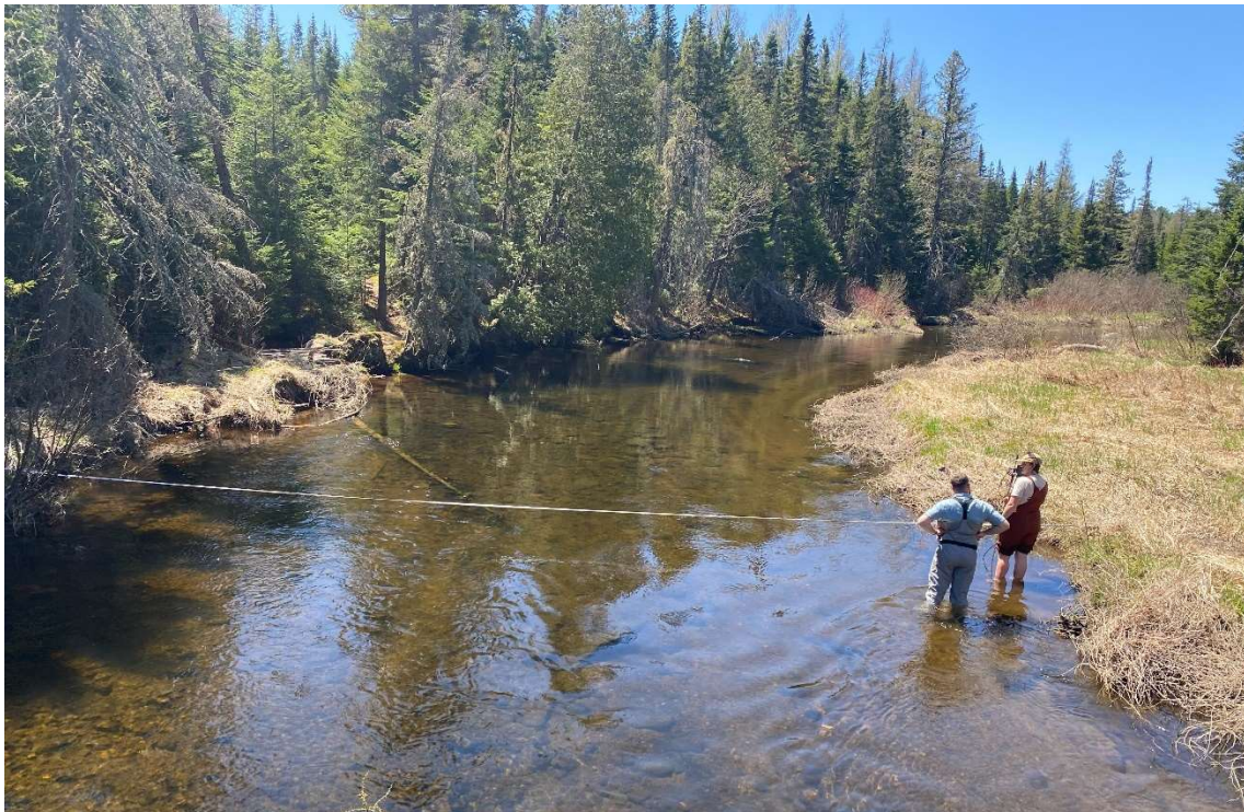
Figure 2. AWI Research Associate, Lija Treibergs, teaching an AWI Seasonal Research Technician and Paul Smith’s College undergraduate student how to measure discharge using an acoustic Doppler velocimeter at the Lower Chubb River site.
