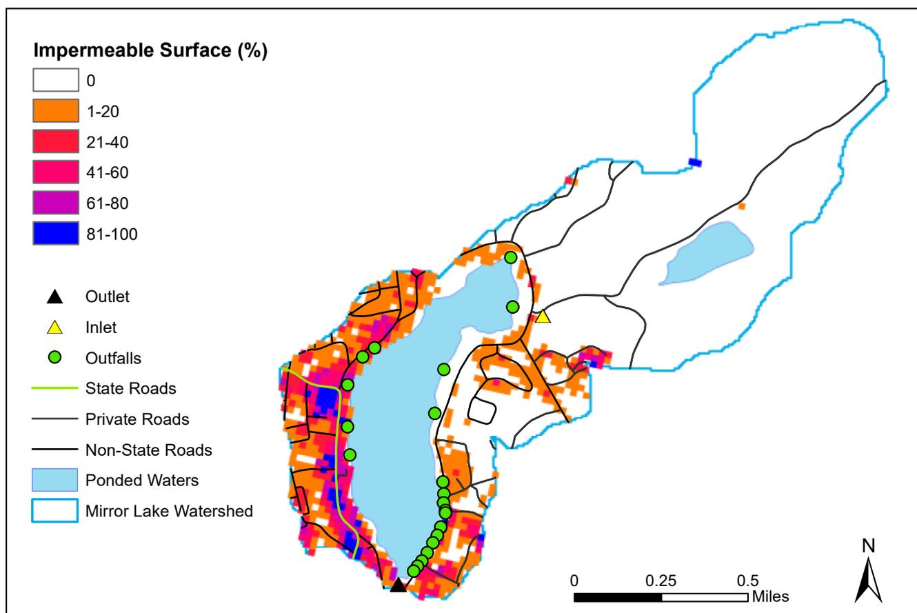
Figure 2. Distribution of impermeable surfaces and stormwater outfalls within the Mirror Lake watershed as of 2016. Many of the outfalls along the southeast side of the lake are no longer in place.
